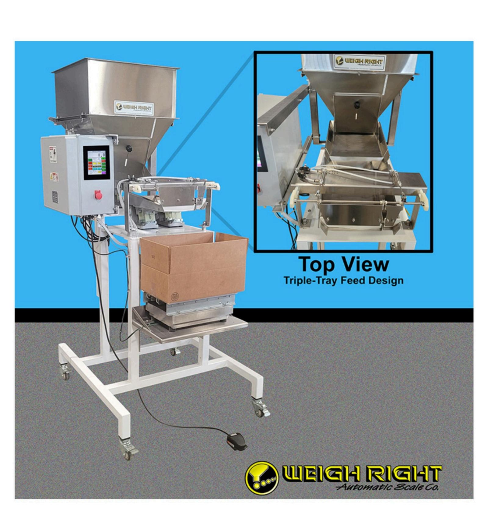
**Shown Above: The G-50-E Direct Fill Scale** featuring a triple-tray feed design.
